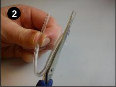
Cut a taper into one end of the new tube using scissors. Some tubes come pre-tapered.
