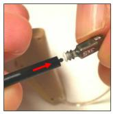
Take a new wax trap from the pack. On the empty end of the applicator stick is a barbed protrusion. Press this into the wax trap you want to remove.
