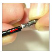
Remove the applicator and the new wax trap will stay in place.
