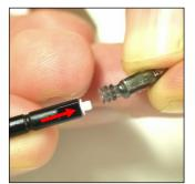
Now flip the applicator around and press the new wax trap in to replace the old one.
