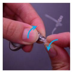
To clean the slim tube, hold the top of the slim tube and turn the hearing aid to detach.
