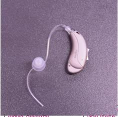
Line up the thread of the slim tube with the adaptor on the aid.
