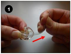
Remove the old tubing by pulling it out of the mould. It may be quite tight.
