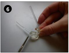
Now cut off the tapered end with a scalpel (or any very sharp knife. Scissors will work but it is difficult to cut close to the end of the mould).
