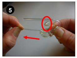
Pull the tube through until you reach the bend in the tube. Notice the top part of the tube is in line with the tip of the prong at the top of the mould (circled in red).
