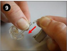
Finally push the hearing aid back onto the tubing.
