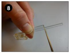
While still holding the old tube over the new, cut the new tube to the correct length. Make it very slightly longer as you can always trim a little more off.
